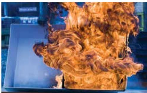
The fire in the box after 4 minutes clearly showing the protective properties of Crystic Fireguard Topcoat 75PA Excel on the left hand side
