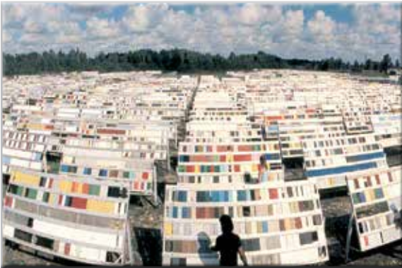
Extreme natural exposure conditions accelerate product weathering, two to three times faster than normal locations.
