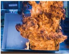
The fire in the unprotected right side box raging after 4 minutes, clearly showing the effective fire protection barrier properties of Crystic® Fireguard 75PA Excel topcoat used in the left side box, when compared to a standard unsaturated polyester topcoat subjected to identical direct flame fire conditions in this simulated test.
