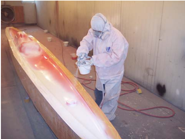
Spray trials with Crystic 253PA successfully demonstrated it to be robust, sag resistant and easy to handle.
