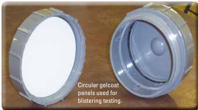
Specially designed test panels at the Atlas Weathering Services Group site in Florida, U.S.A.
