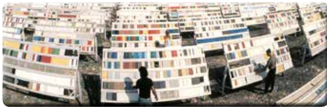
Specially designed test panels at the Atlas Weathering Services Group site in Florida, U.S.A.
