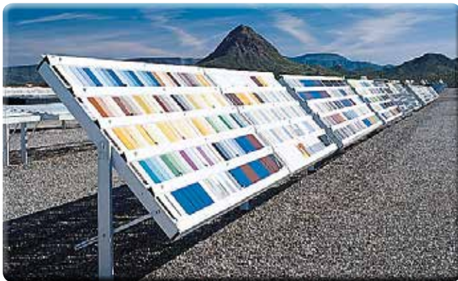
Extreme natural exposure conditions accelerate product weathering, two to three times faster than normal locations.
