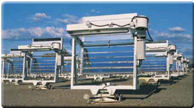
Extreme natural exposure conditions accelerate product weathering, two to three times faster than normal locations.
