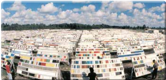
Specially designed test panels at the Atlas Weathering Services Group site in Florida, U.S.A.
