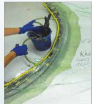
Tauro V8 Spider (Manufactured using Crestapol® 1250LV and Crestabond® M1 Structural Adhesive Range)
