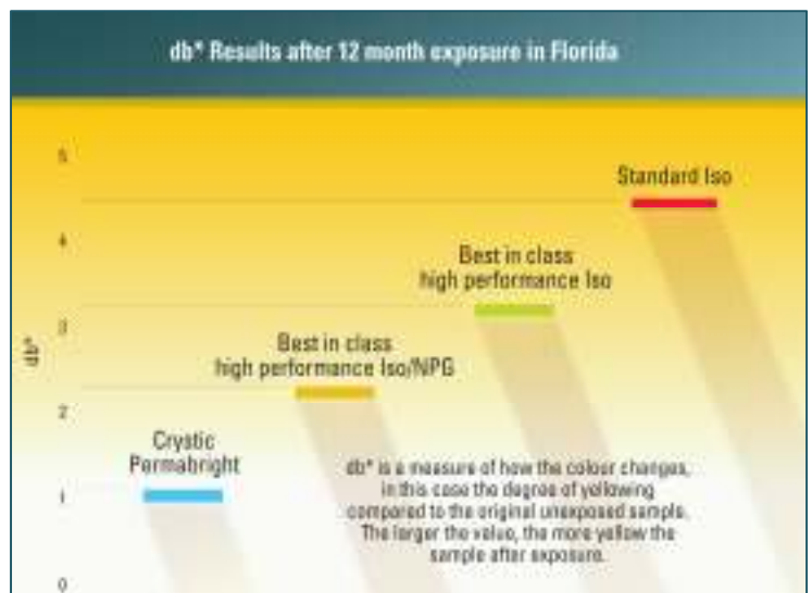
Figure 5: Florida 12 Month Natural exposure delta b* test results which measure the degree of yellowing.
