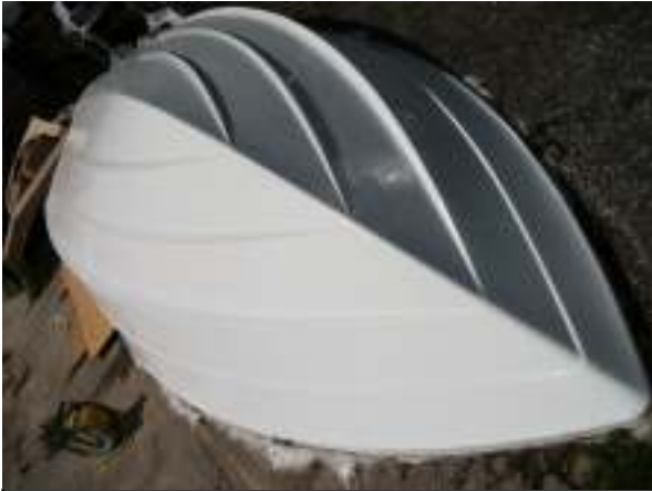
Figure 11. Morgan Sport Boats trial: 20 ft ski boat hull fabricated using new Crystic Permabright gelcoat. A significant improvement in gelcoat gloss and the brilliance of the white colour was noted.
