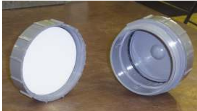
Figure 6: Circular gelcoat panels are placed in the blister test container and then undergo 12 months of testing
