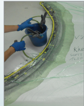
Tauro V8 Spider (Manufactured using Crestapol® 1250LV and Crestabond® M1 Structural Adhesive Range)
