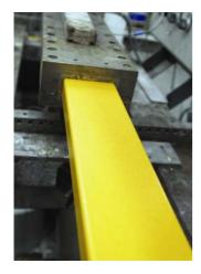
Pultruders benefit from higher productivity with Crestapol1212 resin due to the higher haul off rates possible, even at high ATH filler loadings for demanding building and rail applications where the FRP profile must meet Spanish M1/F0 fire test ratings.
