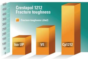
Crestapol 1212 Fracture toughness V's Iso UP and VE resins.
