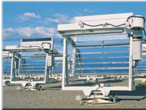
Extreme natural exposure conditions accelerate product weathering, two to three times faster than normal locations.
