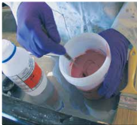
Thoroughly stir in the catalyst to ensure uniform catalysing of the mixture
