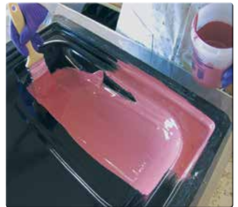
Brush (or spray) onto mould ensuring any trapped air is removed
