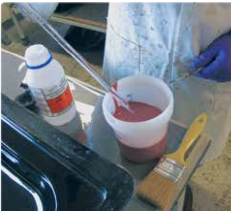
Accurately measure 2% catalyst and add to Crystic Mouldguard
