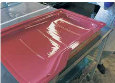
Fully coat the mould ensuring no dewetting or voids. Flange areas should also be coated. Leave to cure before storage.
