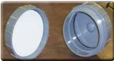
Circular gelcoat panels used for blistering testing.
