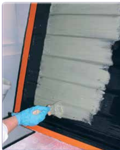
The Crystic Crestacoat 5000PA can then be applied by brush for smaller areas.
