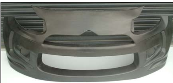
Photo 2: Replacement Carbon-Kevlar composite front bumper
