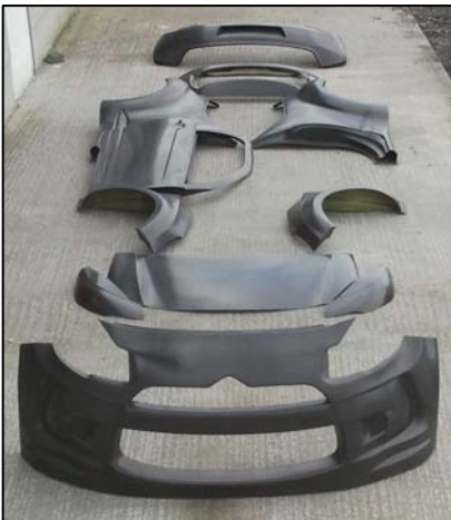
Photo 1: The 11 replacement Carbon-Kevlar composite body panels
