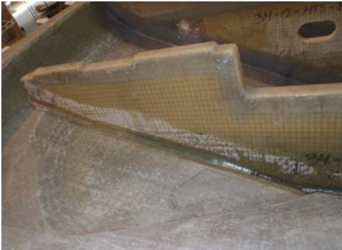
Photo 4 - Schat-Harding FF1200 hull stringer bonded with Crystic Crestomer 1152PA
