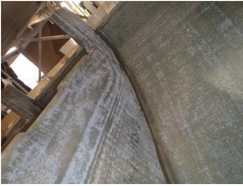
Photo 3 - Schat-Harding FF1200 hull bulkhead bonded in with Crystic Crestomer 1152PA
