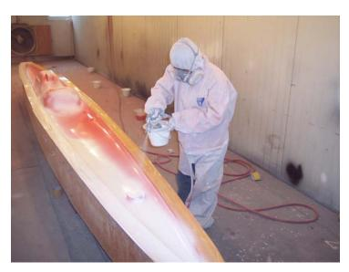
Nelo chose Crystic GC 253PA epoxy bonding spray gelcoat due to its outstanding adhesion to epoxy resin and consistent batch to batch quality.
