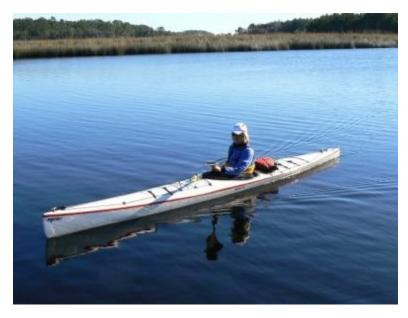
Epic 'Touring' model kayak. The choice of epoxy resin and sandwich core construction used makes them much lighter than most touring kayaks.
