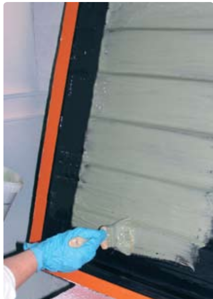
The Crystic Crestacoat 5000PA can then be applied by brush for smaller areas.
