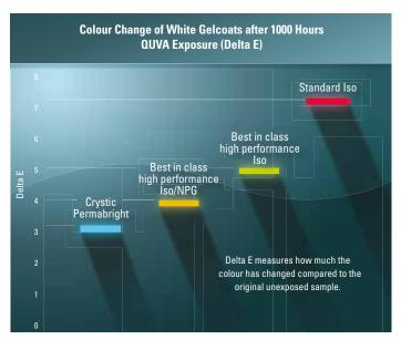
This is an accelerated weathering test which can be used as an indication of performance.
