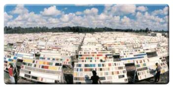
Specially designed test panels at the Atlas Weathering Services Group site in Florida, U.S.A.
