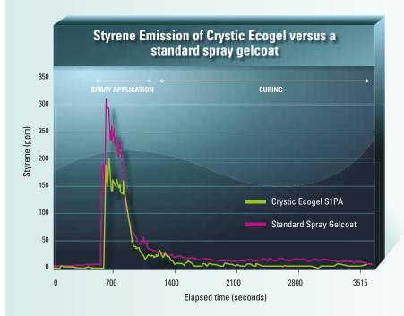
Tests show Crystic Ecogel S1PA has a much lower VOC emission for both the dynamic phase (airless spray) and static phase (gelation) than a standard spray gelcoat
