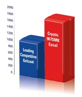
The graph demonstrates 967SMK Excel provides significantly better thermal shock resistance than a leading competitor gelcoat.
