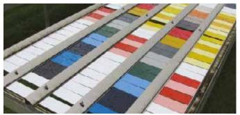
PANELS IN FLORIDA - Extreme natural exposure conditions accelerate product weathering, two to three times faster than normal locations.
