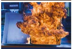
The fire in the box after 4 minutes clearly showing the protective properties of Crystic Fireguard Topcoat 75PA Excel on the left hand side
