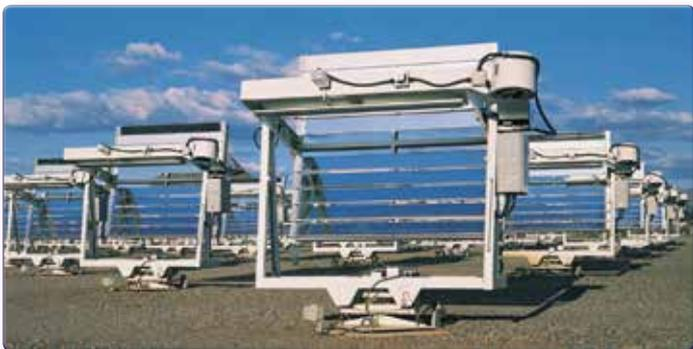
Extreme natural exposure conditions accelerate product weathering, two to three times faster than normal locations.
