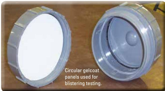
Circular gelcoat panels used for blistering testing.
