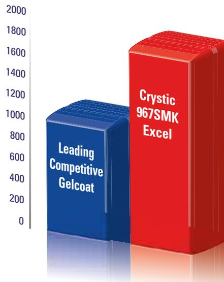
The graph demonstrates 967SMK Excel provides significantly better thermal shock resistance than a leading competitor gelcoat.
